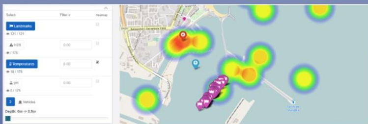
CAF representing multiple data, with vehicles, their heading, landmarks and temperature
